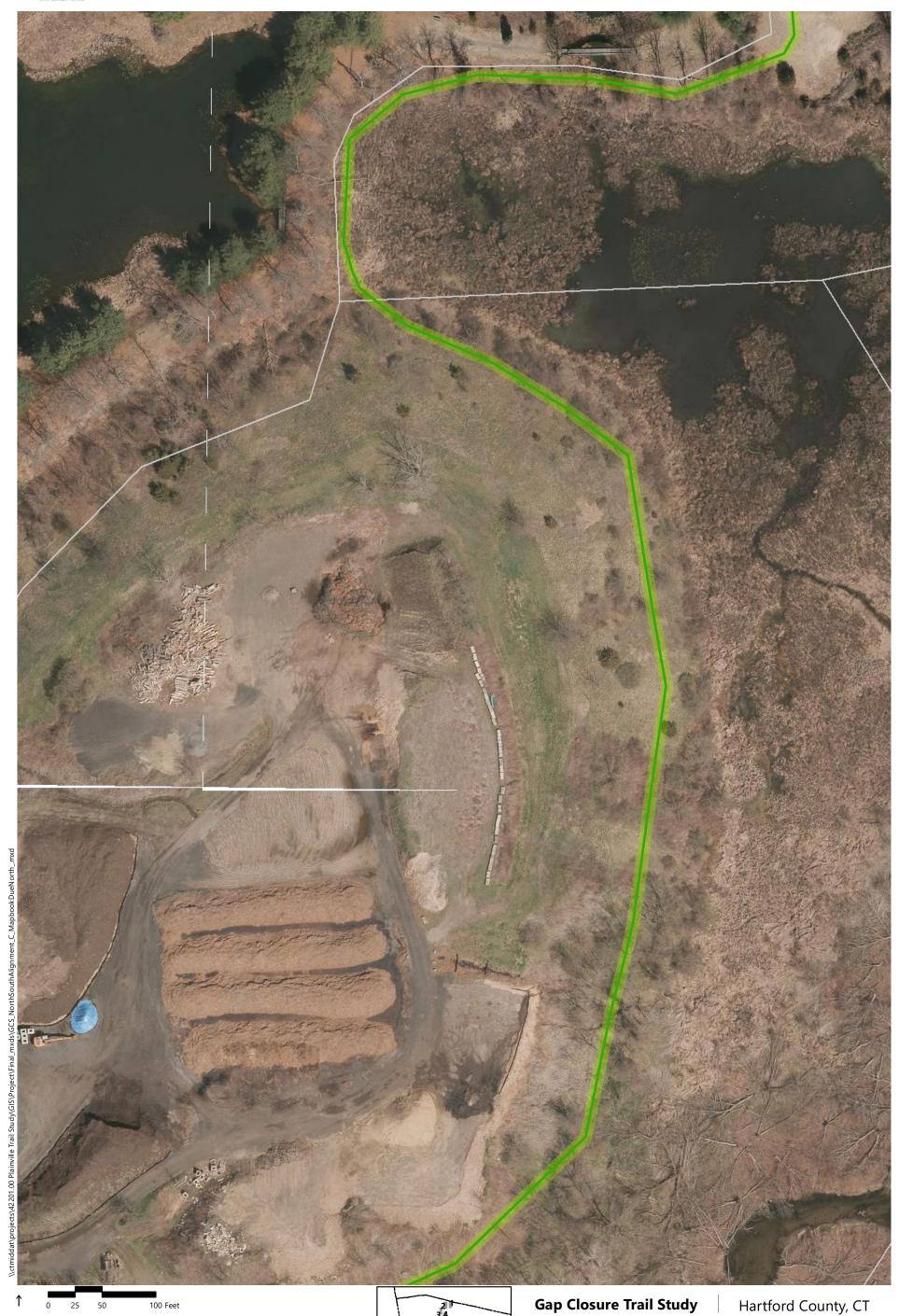
Alignment C Alternatives10-12' Bituminous multi-use trail
